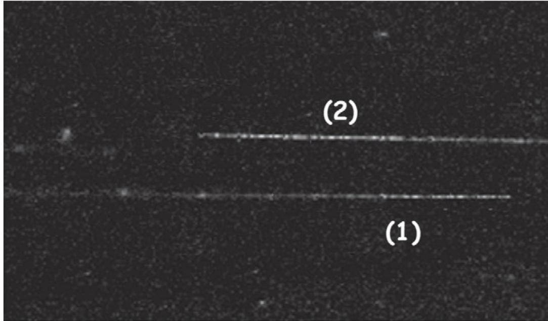
**Fig. 2.** Online display of two simultaneous tracks entering the sensor from opposite sides (100 MeV electrons coming from the right). Track entering from sensor surface (1) and from sensor back (2).
