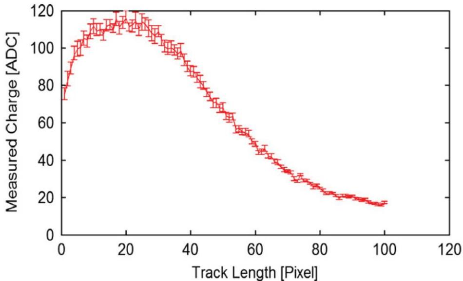
**Fig. 9.** Charge collection efficiency profile for MT9V011 sensor.
