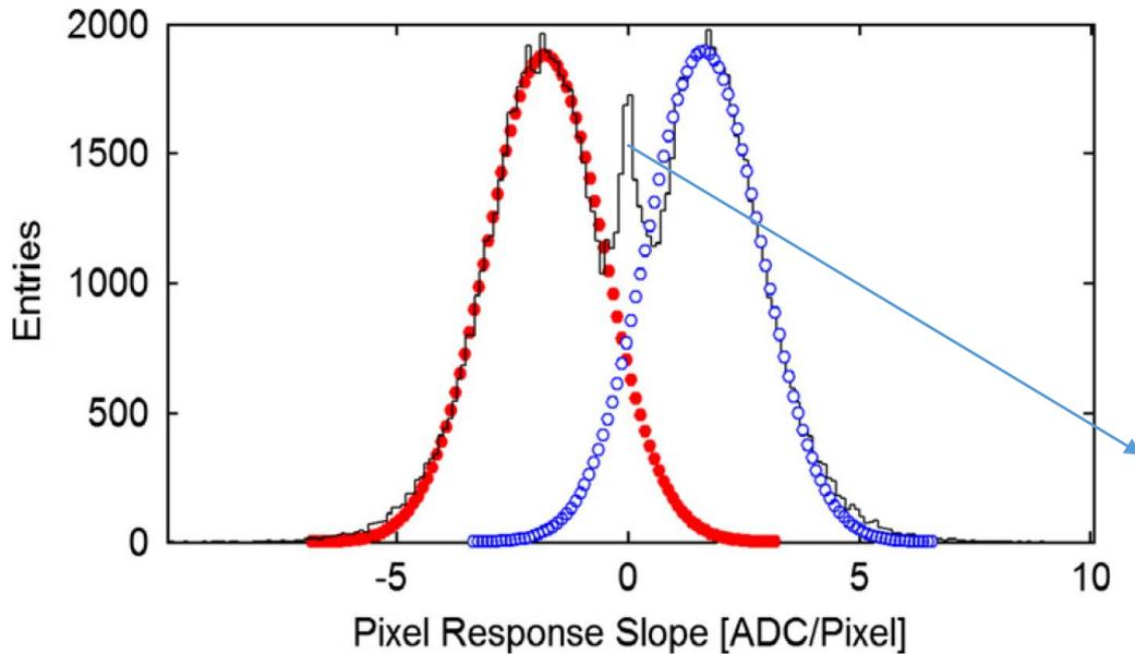
Fig. 7. Distribution of the Pixel Response Slope measured with tracks entering from the sensor surface (filled circle) and from the sensor back (open circle).
