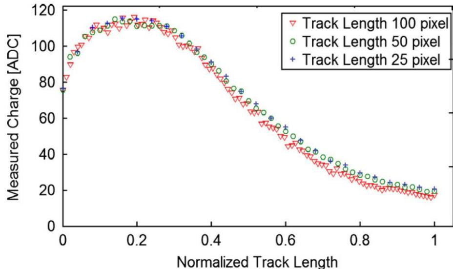
**Fig. 11.** Charge collection efficiency profiles measured with different track lengths.
