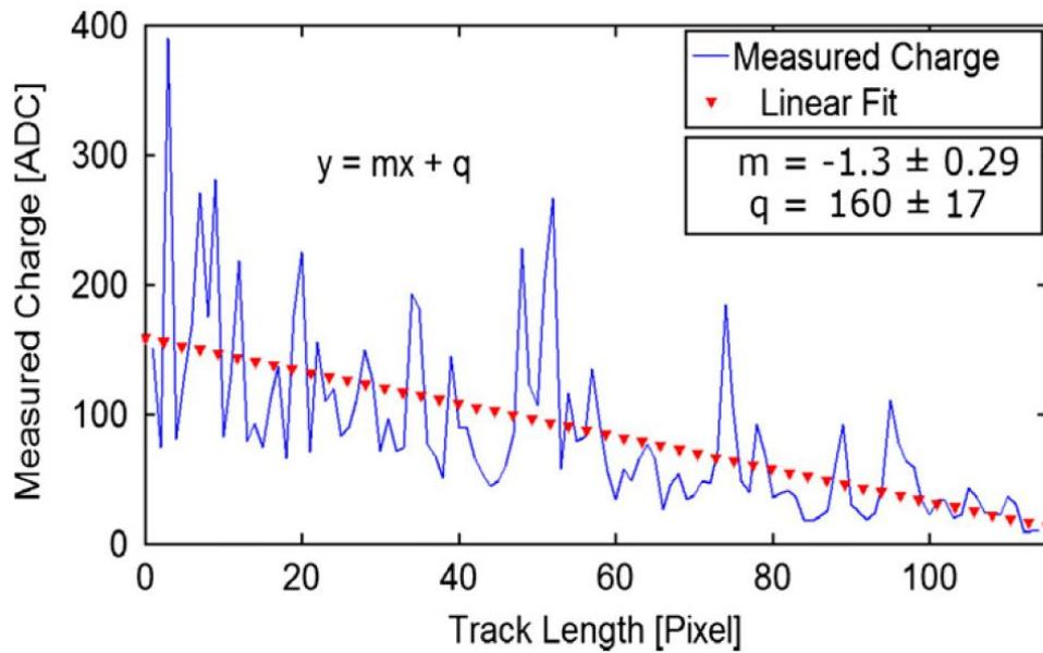
Fig. 6. Pixel response of one track entering from the surface with linear fit.
