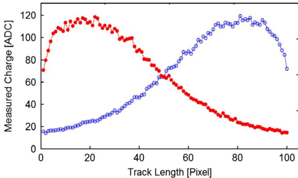
**Fig. 10.** Charge collection efficiency profiles measured with tracks entering from the sensor surface (filled circle) and from the sensor back (open circle).
