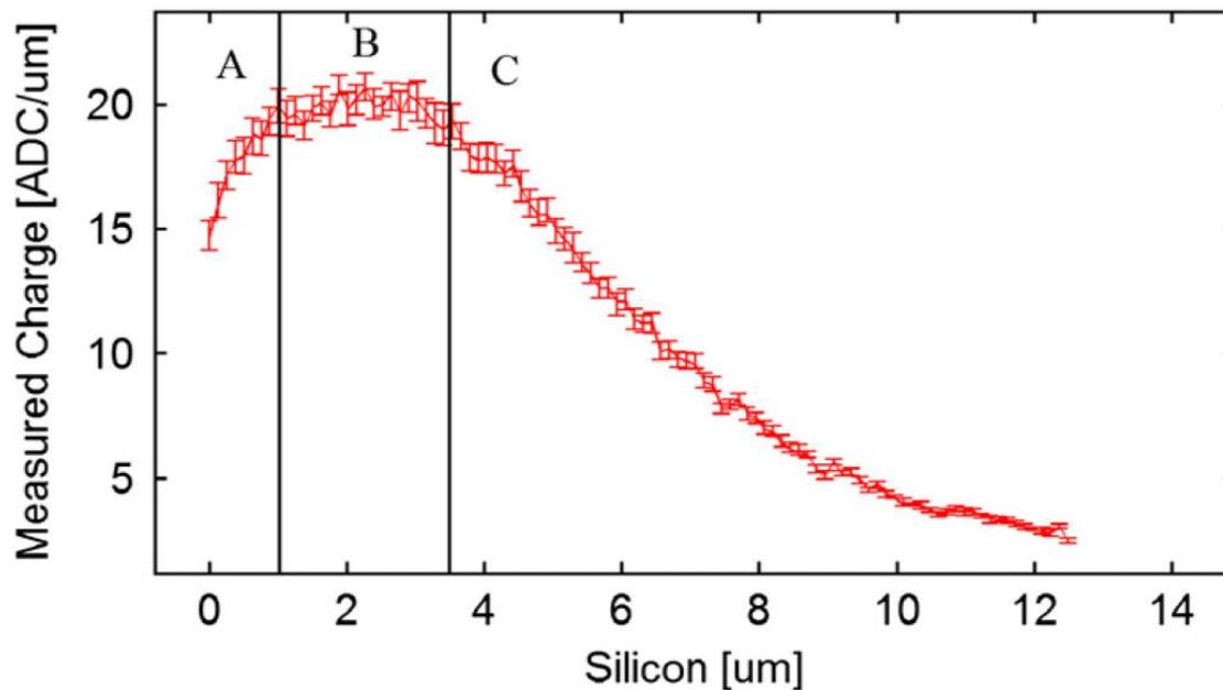
**Fig. 13.** Charge collection efficiency profile for MT9V011 sensor.
