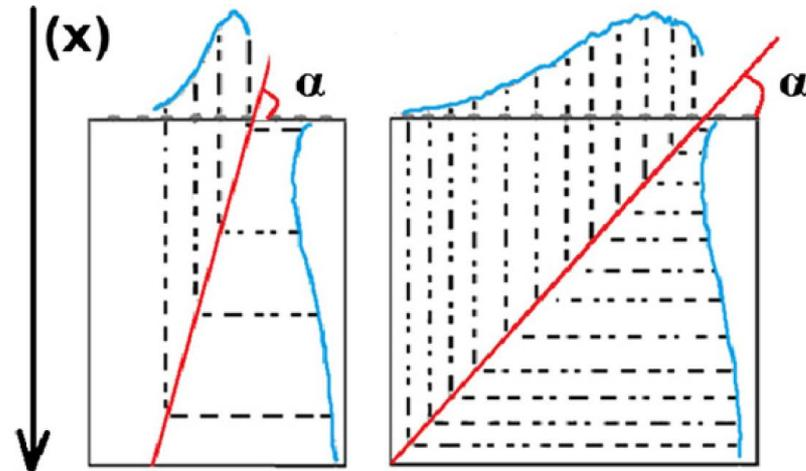
**Fig. 12.** Scheme of charge collection efficiency profile measurement using grazing particles.
