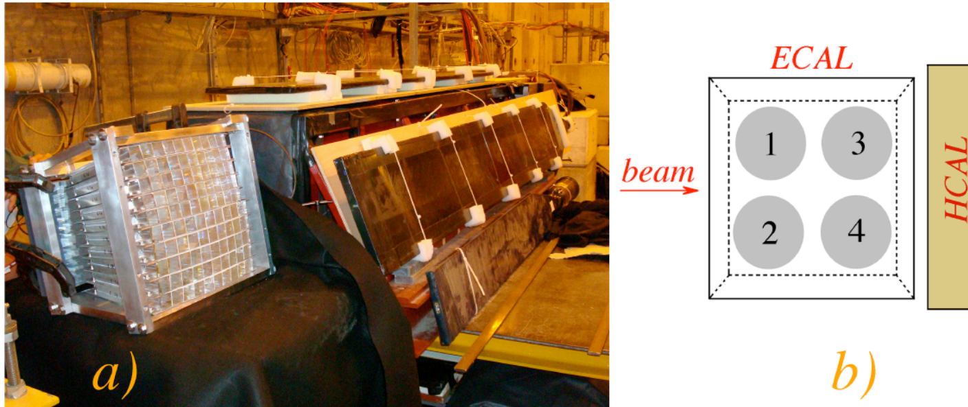
Figure 15: The calorimeter during installation in the H4 test beam, which runs from the bottom left corner to the top right corner in this picture. The 100-crystal BGO matrix is located upstream of the fiber calorimeter, and is read out by 4 PMTs on the left (small end face) side.
