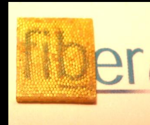
Pixels diameter 350 \mu\text{m} Array surface 10 mm x10 mm
