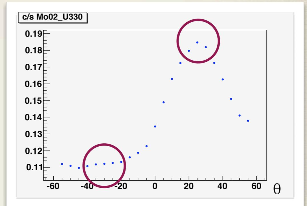
A figure of merit for separation power is the ratio of C/S at the Čerenkov angle and C/S at the anti-Čerenkov angle
