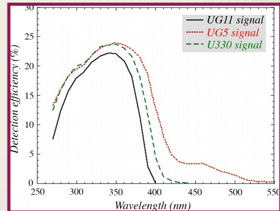
Detection efficiency of light exiting the crystal including optical transmission of the filter and the cookies and QE of the photocathode (Hamamatsu R8900U-100 SBA (36% QE))
