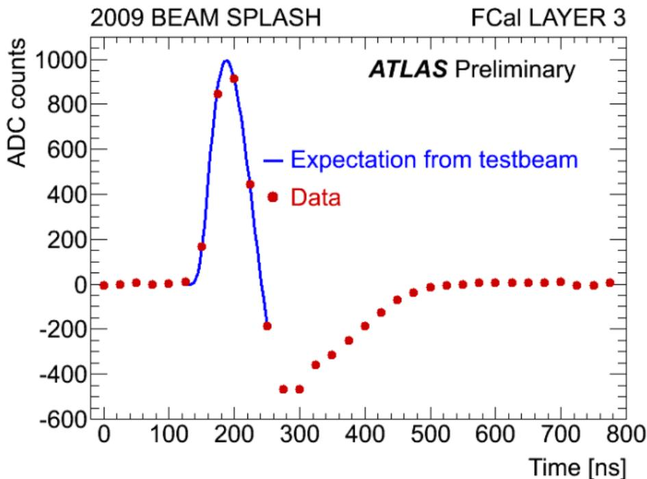
*Example of a signal pulse in the second hadronic layer recorded in beam splash data.*
