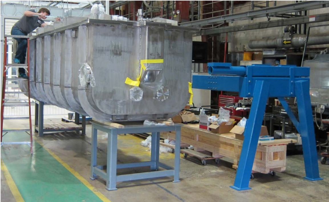
Figure 3.35: The finished vessel assembled at Argonne. The vessel is now being prepared for cryogenic testing.
