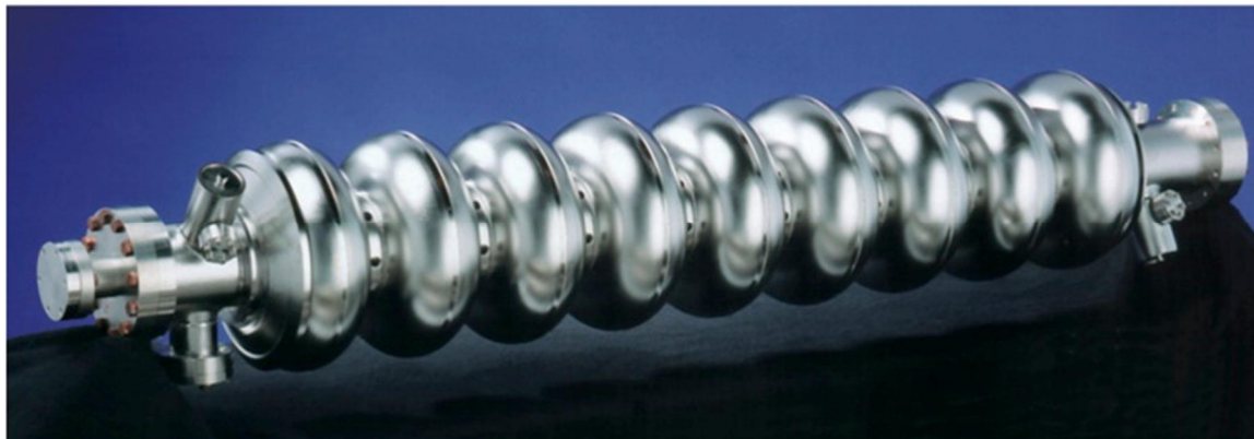
Figure 6-8. LCLS-II baseline cavity: TESLA style 9-cell niobium cavity.
