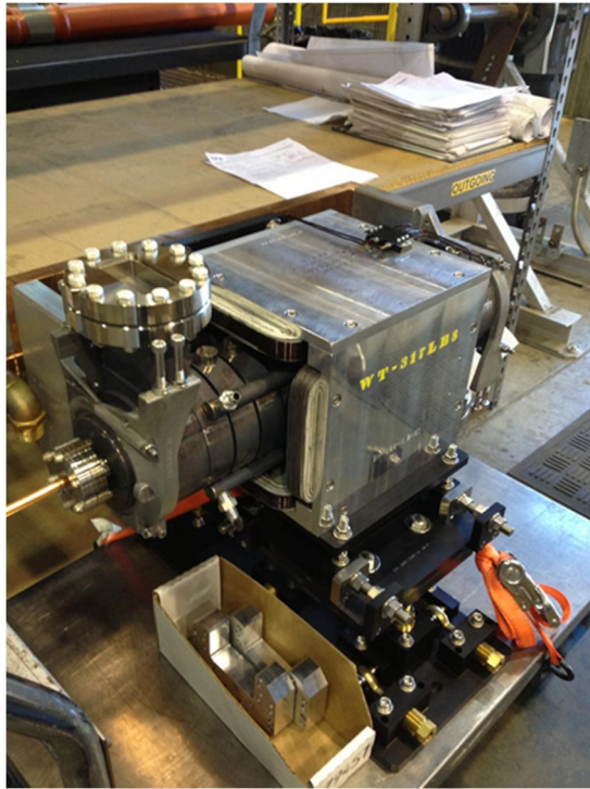
Figure 5-58: Photo of Completed LCLS-II S-band TCAV with steering coils wrapped around it to save beamline space
