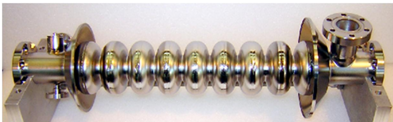
Figure 6-30. 3.9 GHz 9-cell cavity, showing end-groups.
