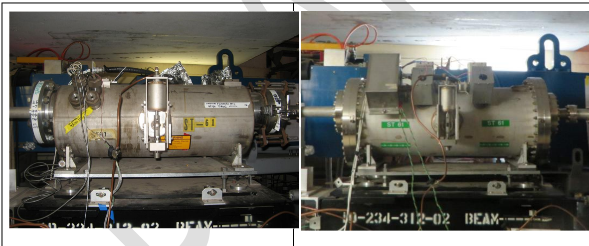
Figure 5-69. Old (left) and new (right) versions of ST61 stopper
