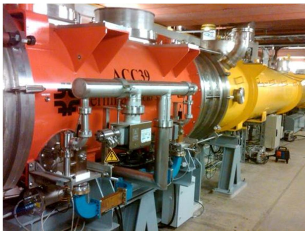
Figure 6-26. 3.9 GHz cryomodule built at Fermilab and installed in the FLASH facility at DESY
