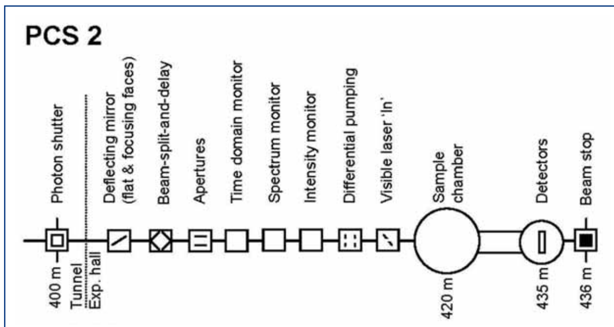
Figure 6.4.36 Schematic layout of the PCS 2 instrument at the SASE 3 beamline. For this instrument diagnostics will be placed entirely upstream of the sample. The distance sample-detector can be varied.
