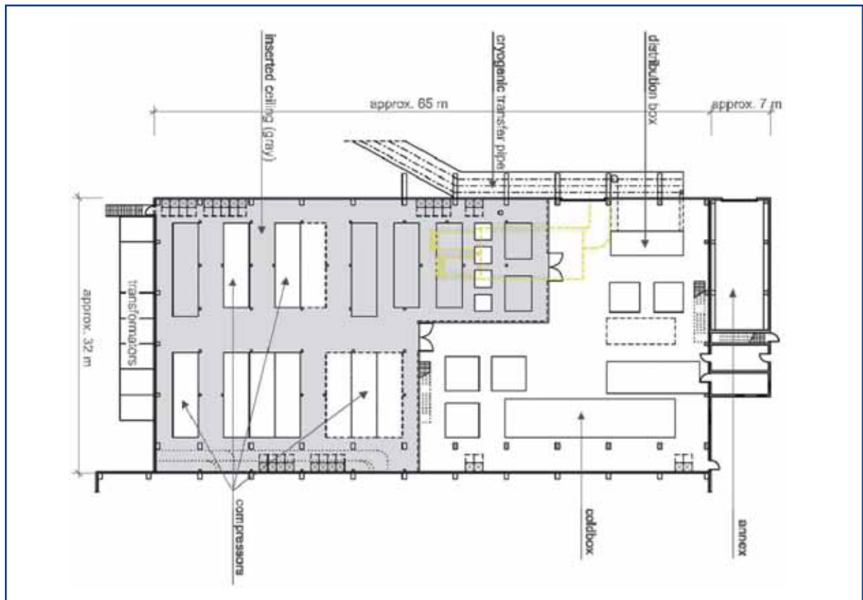
Figure 7.1.8 Ground plan of the XFEL cryogenics hall. The dimensions of the hall are about 72 m x 32 m with a height of about 14 m.
