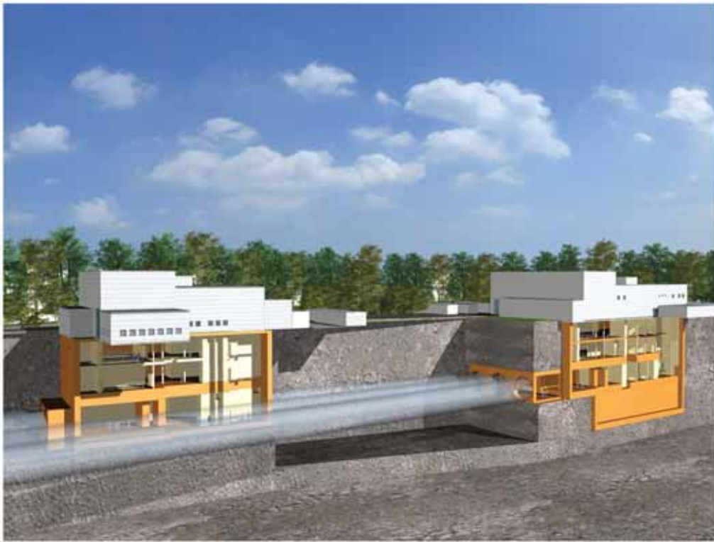
Figure 7.1.24 Three-dimensional view of the shaft complex XS1 and XS5 at the XFEL site Osdorfer Born.
