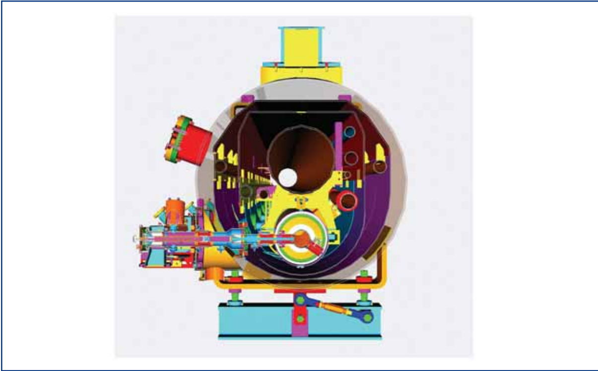
Figure 4.2.15 Cross-section of a type-3 cryomodule.
