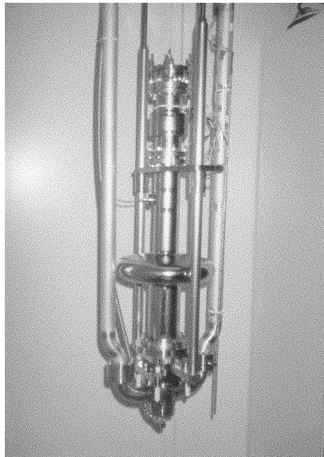
Figure 8.50: One-third scale Niobium round-cell crab cavity mounted on a test stand.
