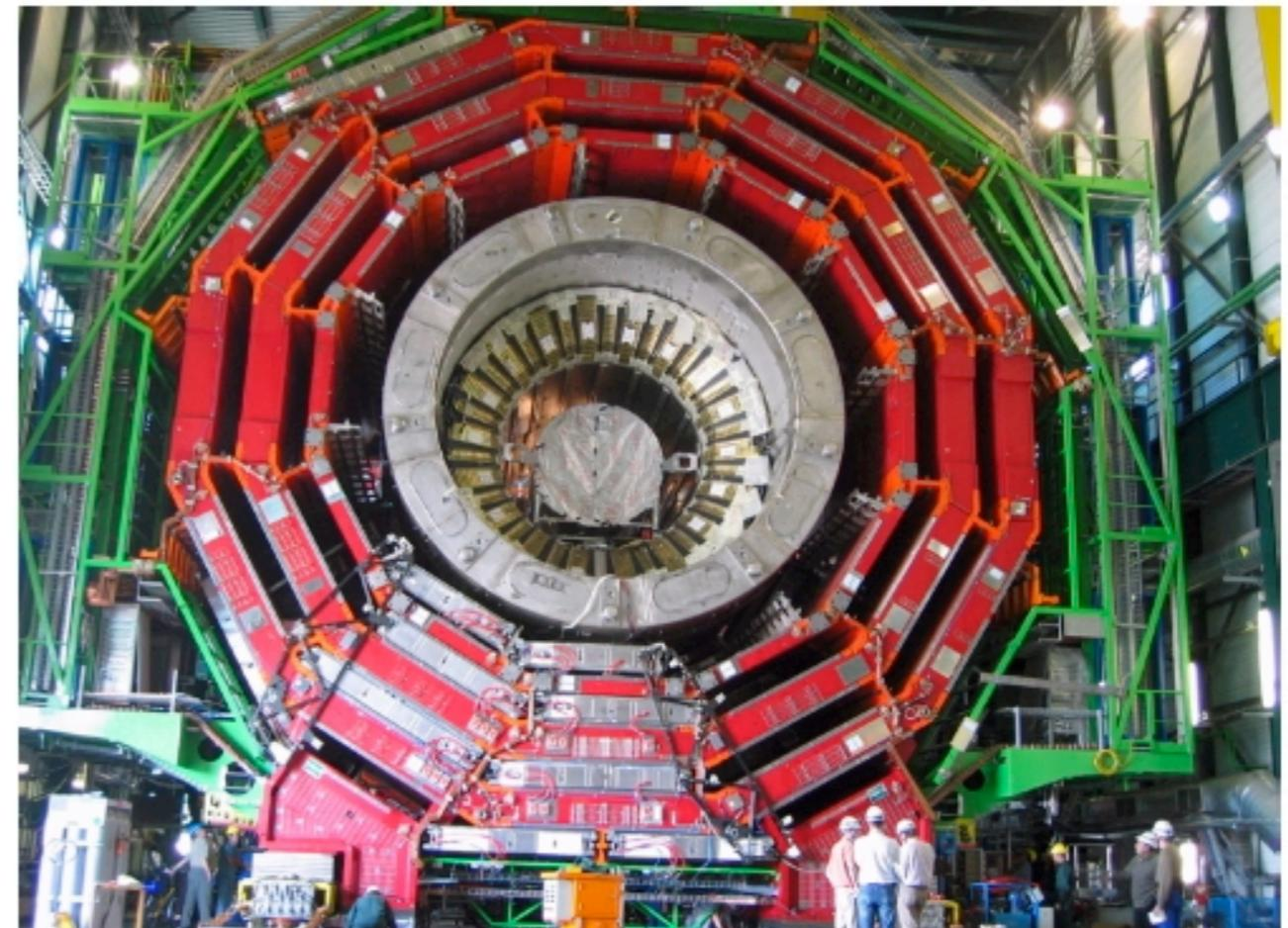
The CMS detector is being closed. The situation viewed from the -end (early last week) shows the YB-2 wheel (and YB-1) closed with the DT+RPC packages, the Barrel HCAL and the Tracker tube installed. Not visible are two SM modules installed at the +end, and the endcaps systems.
