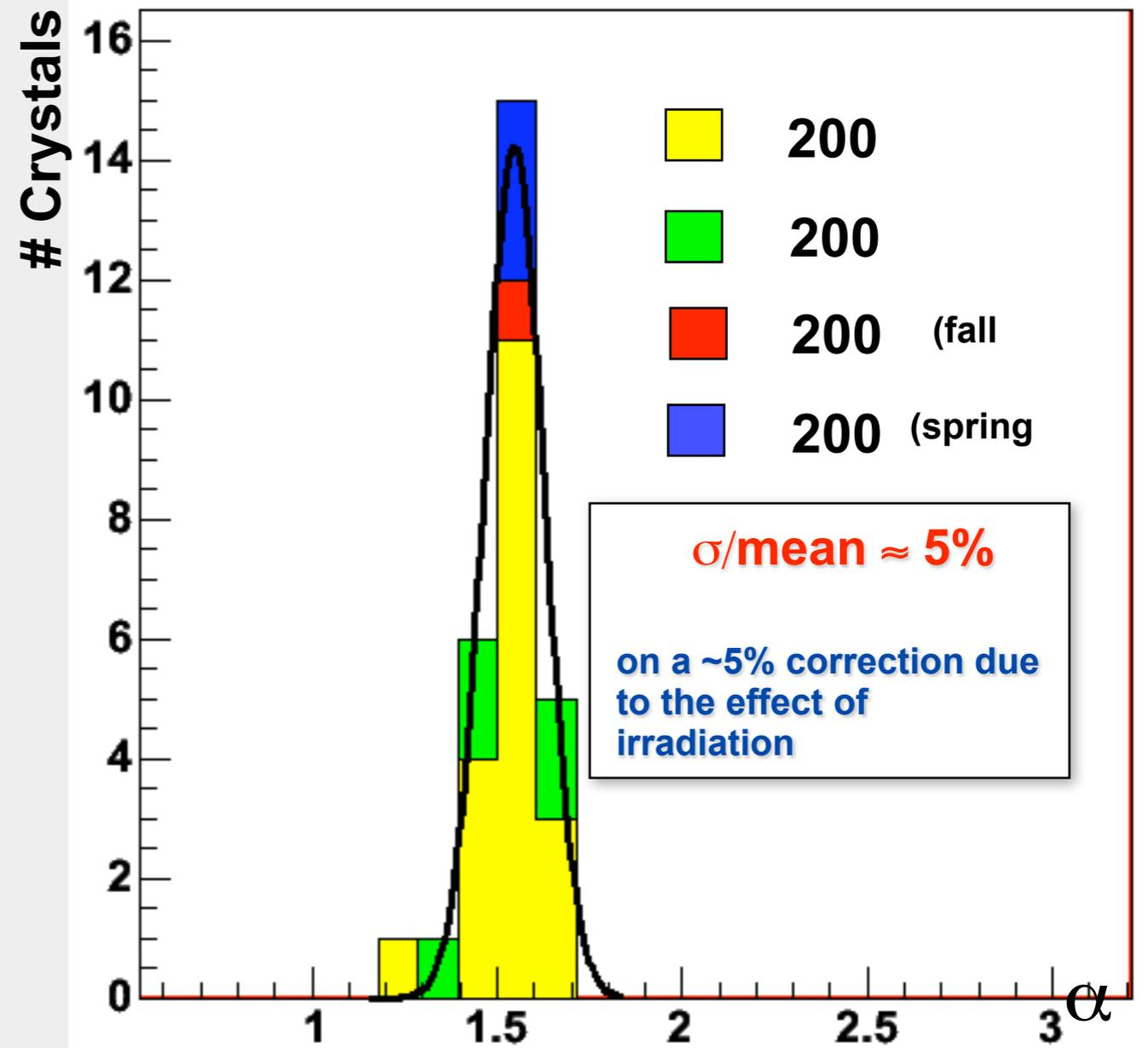
⇒ Coefficient for crystals have relatively small dispersion.
