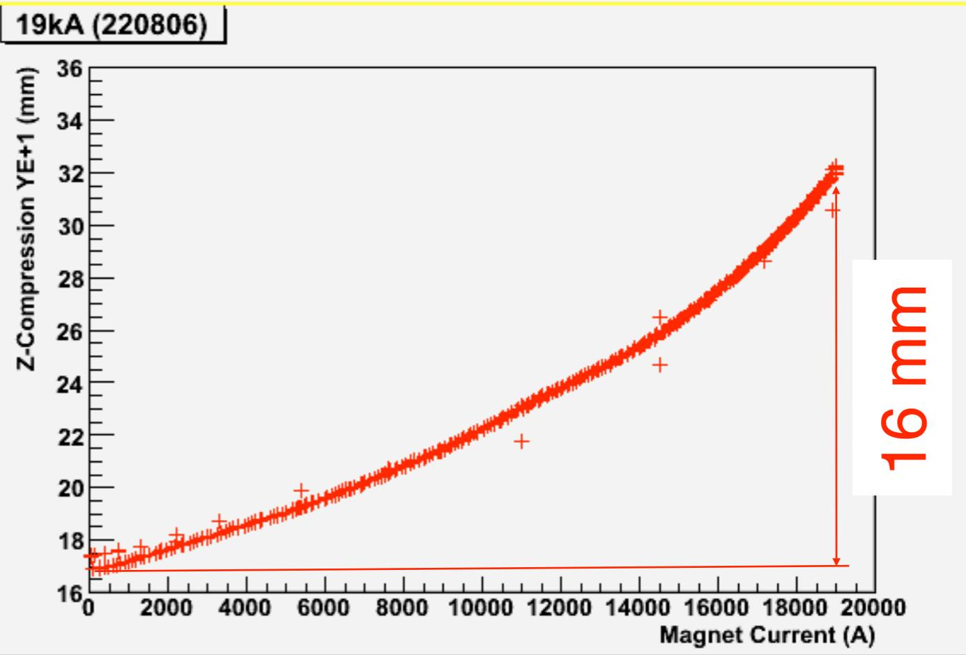
Due to the 10,000 tons magnetic attraction force, the Nose of the 600mm thick YE1 disk moves toward IP by 16mm!
