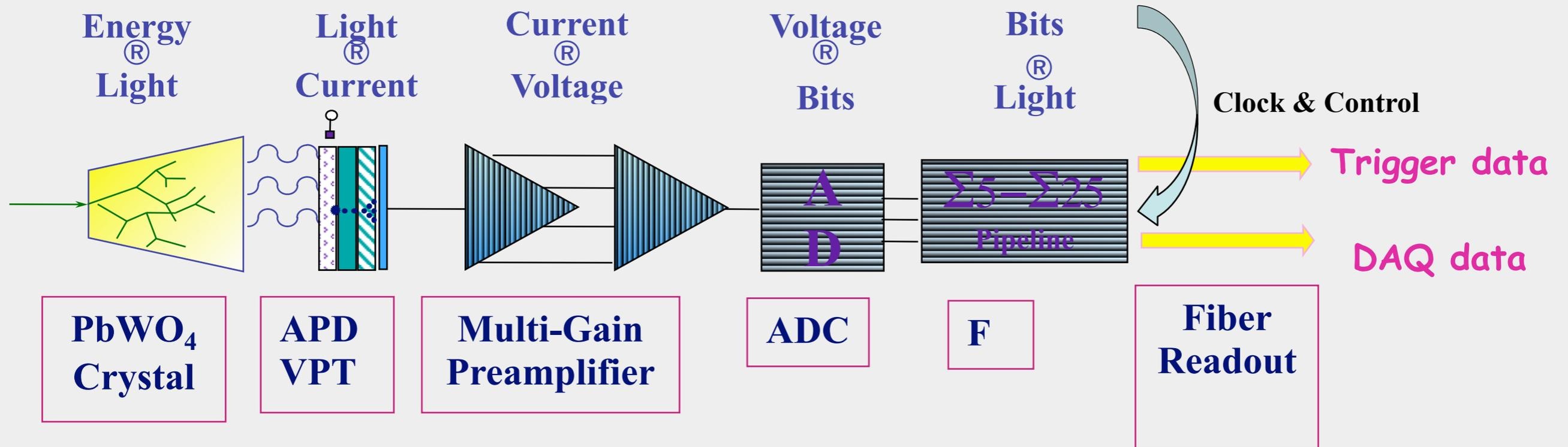
Front-End electronics block diagram: light to light readout chain
