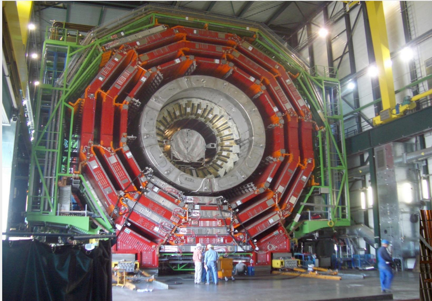
Both –end muon wheels are closed: airpads, grease pads + "proximity capture" hydraulic jacks
