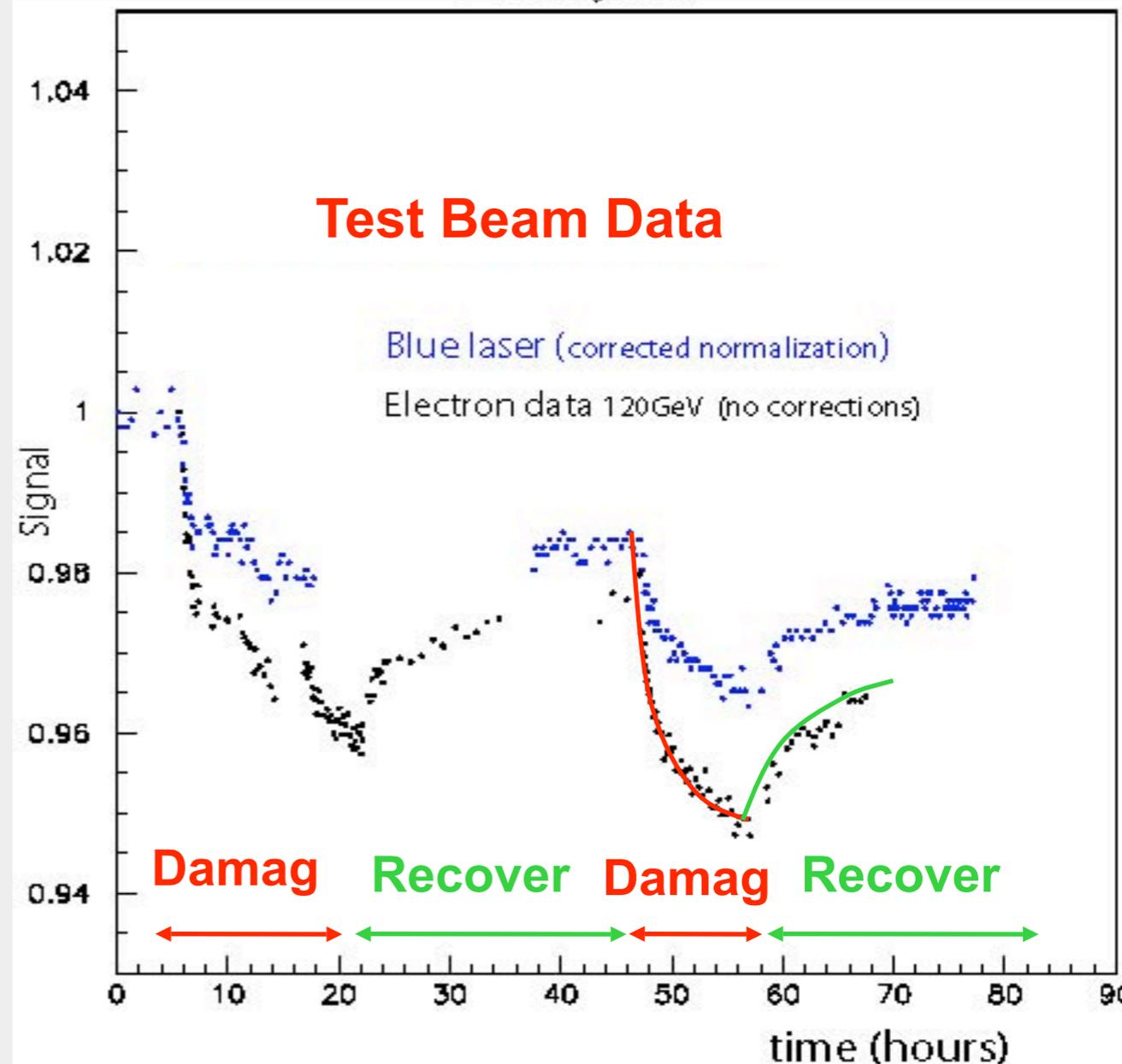
⇒ **Damage-recovery cycle in sync with the ~12 hour LHC fill cycle**
