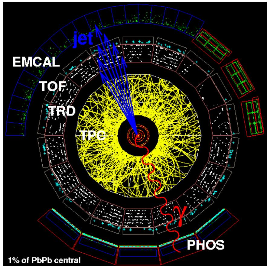
combination of PHOS, EMCAL, particle tracking & Id. allows to get jet trigger, energy loss, particle composition, transverse structure & fragmentation function down to low  $p_t$
