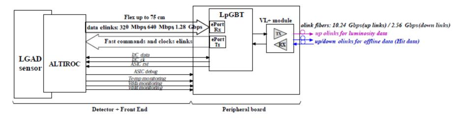
Different data and control lines between ALTIROC and peripheral electronics through the flex (~25 to 75 cm length):
