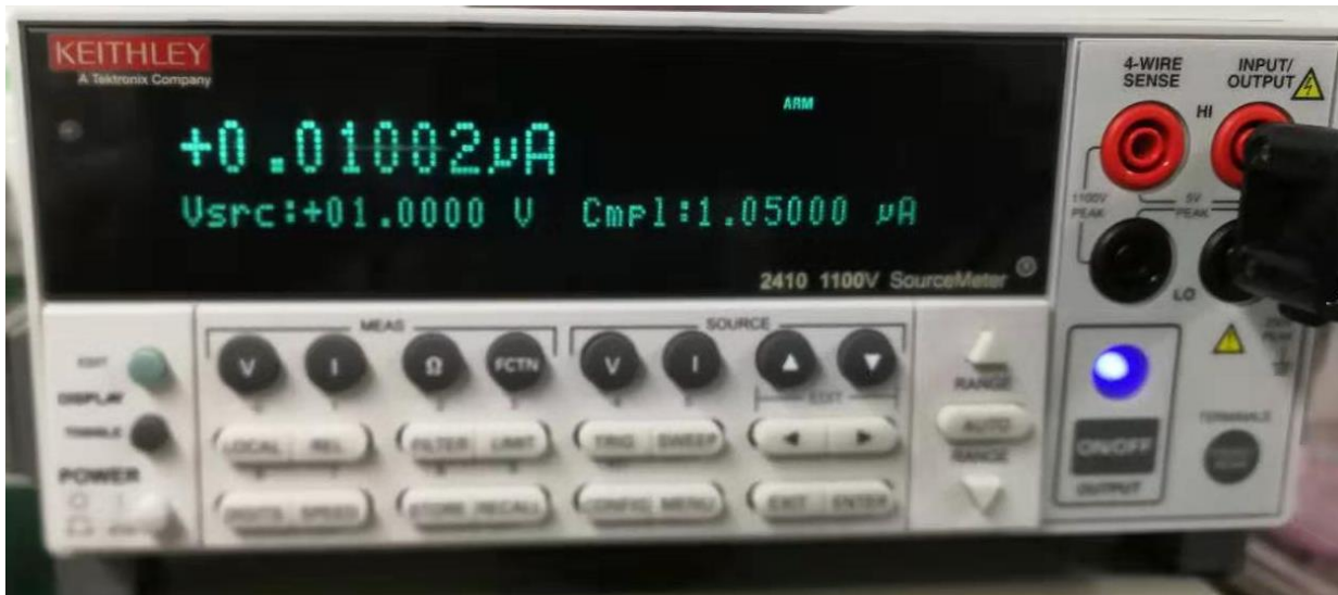
Fig : Since a resistor of 1\text{M}\Omega is inserted, 1\text{V}/1\text{M}\Omega = 0.01 \mu\text{A} is the nominal current.
