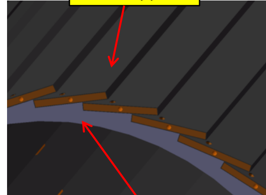
End Ring (CFRP): fix the end of local support by bolting connection.
