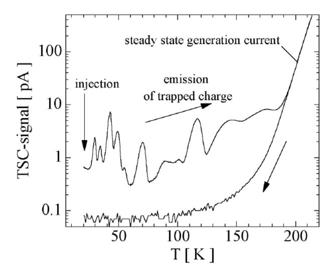
Figure 4.15: Typical TSC spectrum of a detector irradiated with  $\Phi_{eq} = 1 \times 10^{13} \,\mathrm{cm}^{-2}$ . (sample M20713;  $\beta = 0.183 \,\mathrm{K/s}$ ; 30 s injection at 20 K (1.7 mA); 100 V; after 100 min annealing at room temperature)
