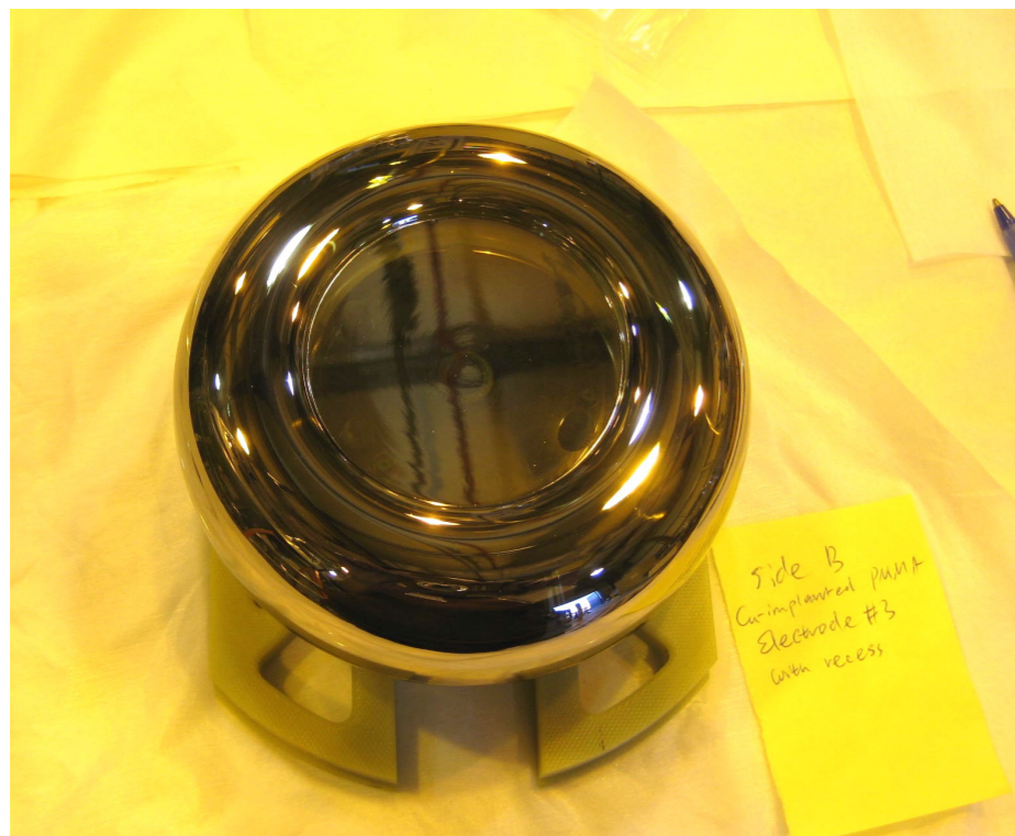
Cu ion implanted PMMA electrodes with a mockup cell.
