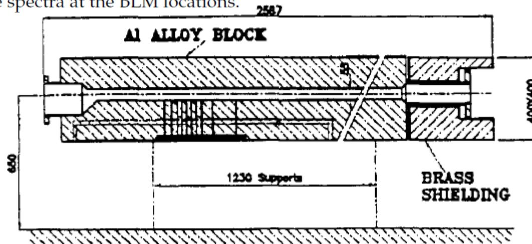
Figure 2: Beam absorber sketch
