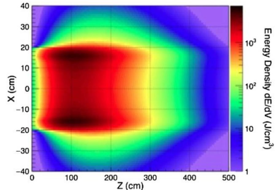
Fig. 2.42. The energy deposition on the beam dump for FCC-ee.
