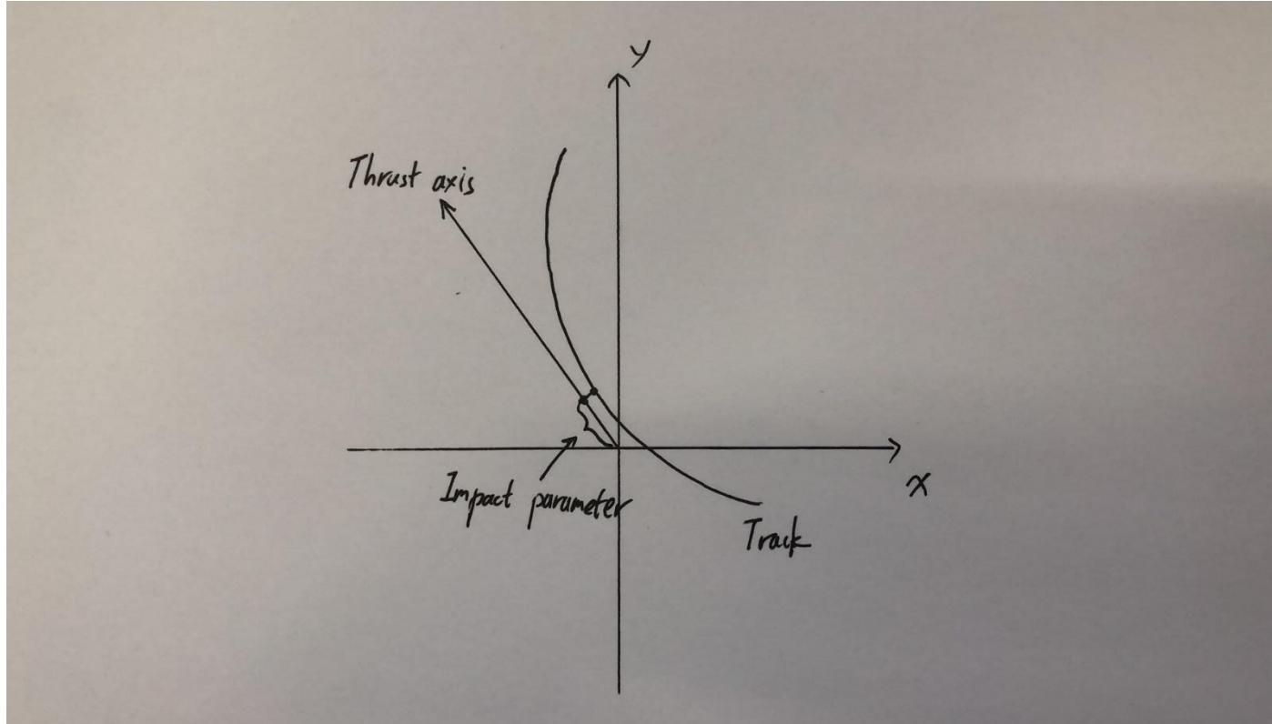
Find the point on the thrust axis closest to the track. The impact parameter is the distance between that point to the IP (I drew in 2D space but calculated in 3D space).
