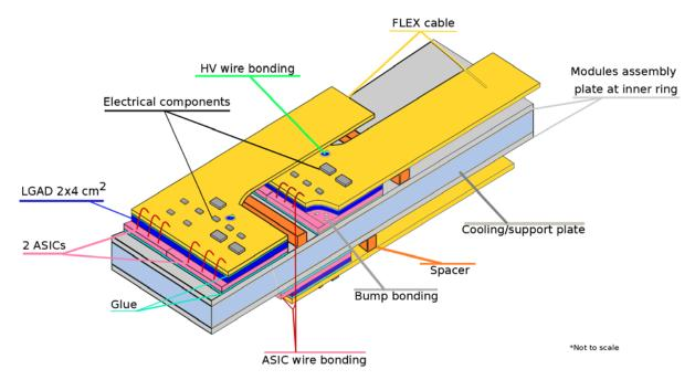
L shape design to reduce the total thickness of the flex cables
