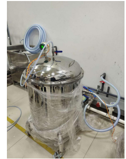
Pressure test (sampling test)
