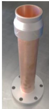
Pumping out pipe
