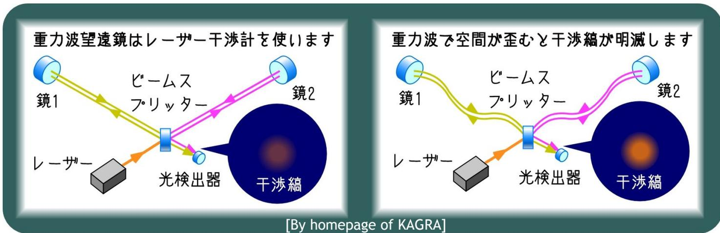
If GWs come to the interferometers, the interfered fringe changes by extending and shrinking the lengths of the arms.
