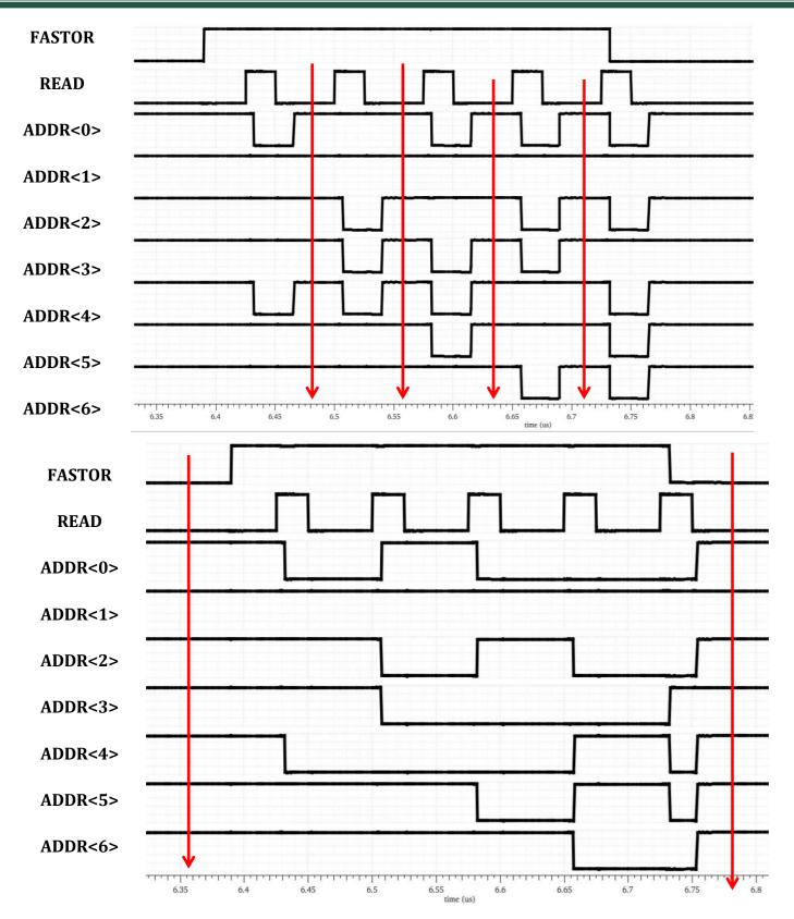
This is the schematic level simulation of FE-I3, the top one connected the pull-up cell without controlling signal, address encoder will be a refresh to the high level before next hit.
