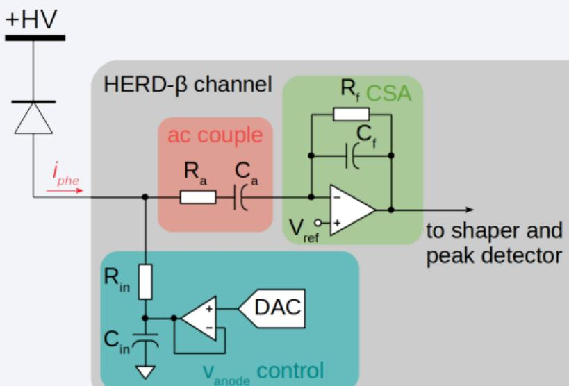
Dynamic Compression of the signal in CSA using MOS cap in feedback.
