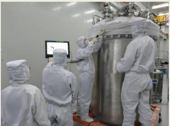
Inner vessel is being put in outer vacuum vessel, which is in water tank.
