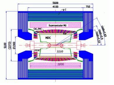
TOF:  $\sigma T = 68(65)$  ps barrel (endcap)
