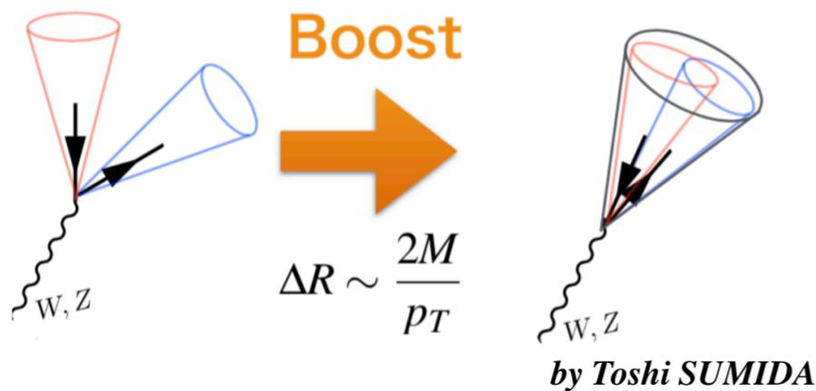
Boosted boson jet: high  $p_T$ , variable  $\tau_1$  and  $\tau_2$  describing jet substructure.
