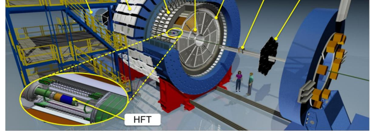
✓ TPC: Tracking, momentum and dE/dx  $\checkmark$  TOF: Time of flight, particle identification
