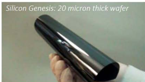
Ultra-thin chip (<50 \mu\text{m} ): flexible with good stability
