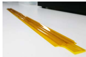
Mock-up ladders made of tape heaters
