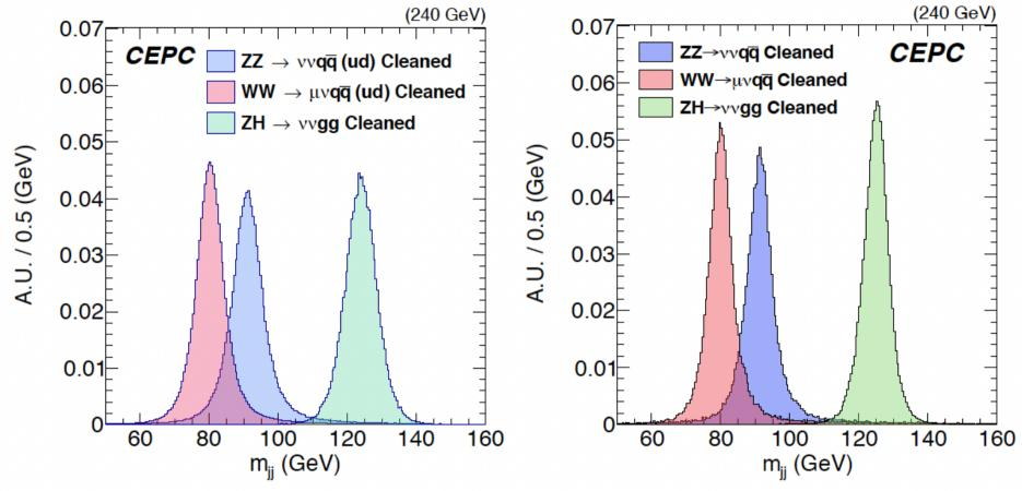
Detector change (usage of high density scintillating glass HCAL): BMR 3.7% → 3.4%;
