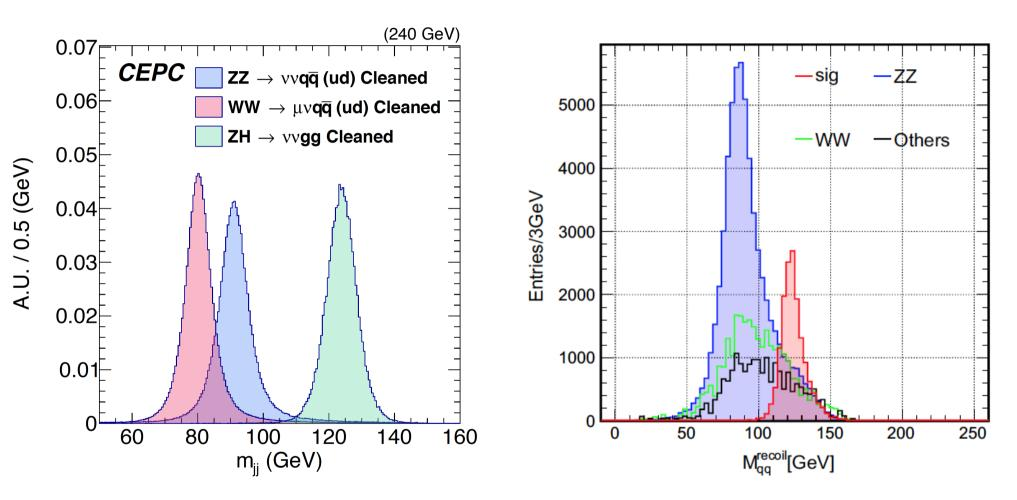
Higgs factory: need BMR < 4% (critical for qqH & qqZ separation using recoil mass to di-jet) Strongly motivated to improve BMR to 3% or even lower, especially for NP & Flavor CDR baseline (left plot): BMR = 3.75%
