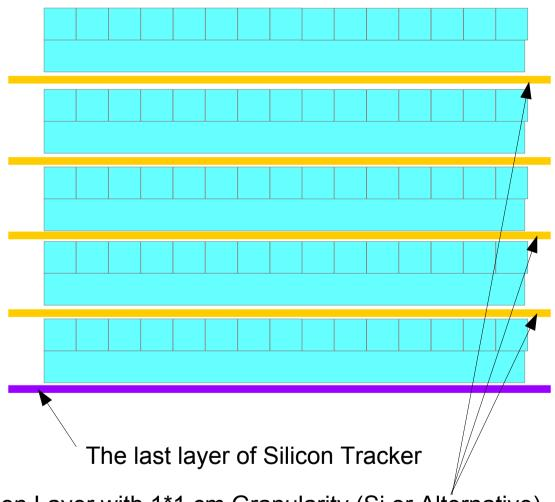
Position Layer with 1\*1 cm Granularity (Si or Alternative)
