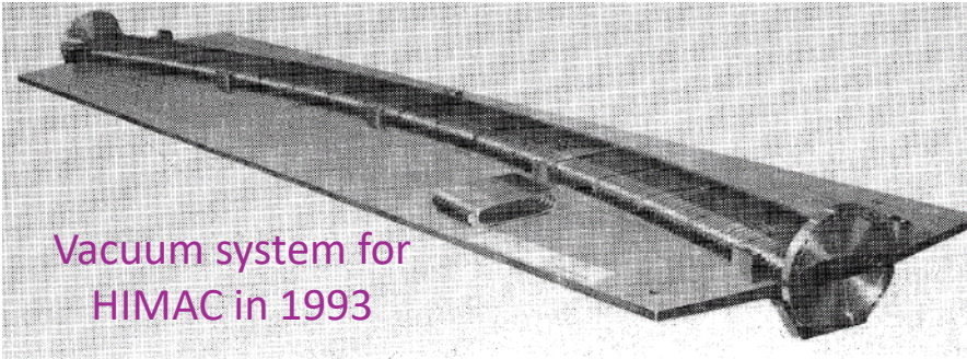
Figure 1a. One section of vacuum chamber set on a steel plate with the same curvature as the bending magnet.
