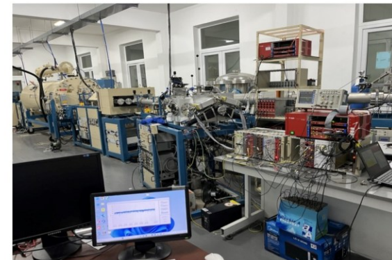
Picture in lab of the detector system and the DAQ connected to Pelletron
