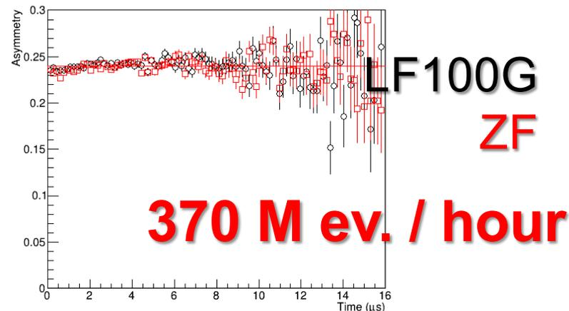
The integrity of the  $\mu$ SR DAQ system was confirmed during the 1MW test operation in Jul. 2018. The above time spectra were obtained in ONE minute.
