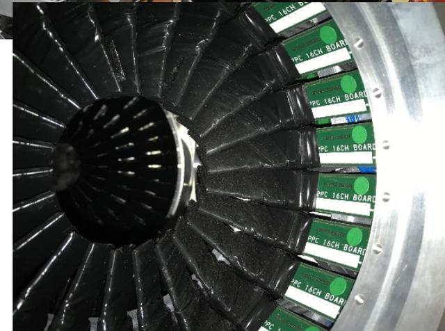
1x1 mm<sup>2</sup> scintillating fibers are aligned in a spiral to meet the  $e^+$  track under high fields.
