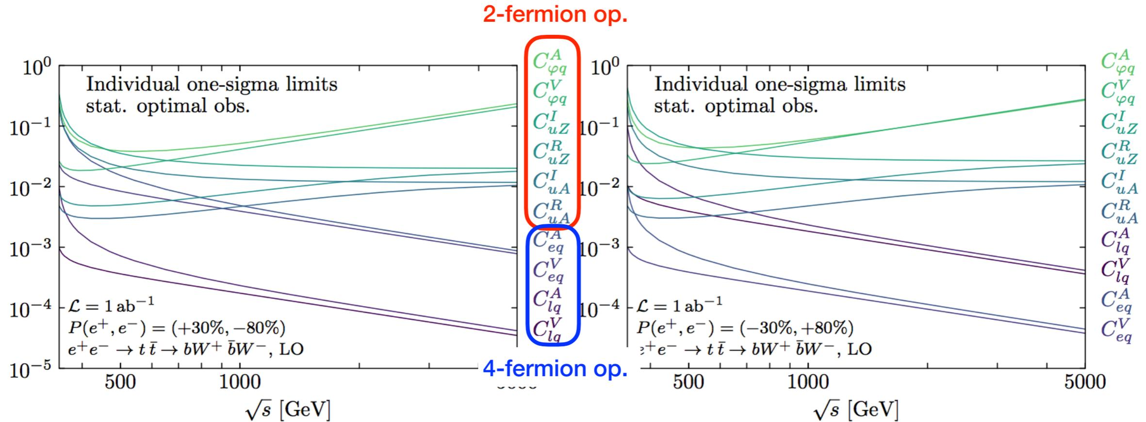
**Figure 16.** Individual statistical one-sigma constraints on the effective operator coefficients as functions of the centre-of-mass energy, for either mostly left-handed and mostly right-handed electron beam polarizations, and a fixed integrated luminosity of  $1 \text{ ab}^{-1}$ . Different integrated luminosities are trivially obtained through a  $(\mathcal{L} [\text{ab}^{-1}])^{-1/2}$  rescaling.
