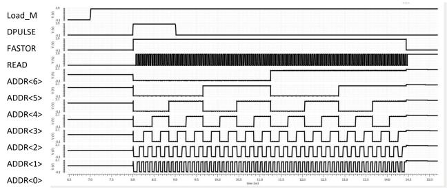
→The simulation shows that everything is fine with the digital injection pulse and mask the pixels.
