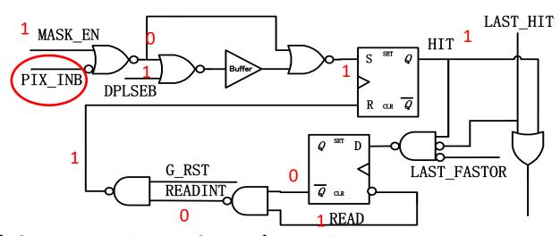
→If MASK\_EN changes from 0→1,it will generate a pulse and record by the circuit.
