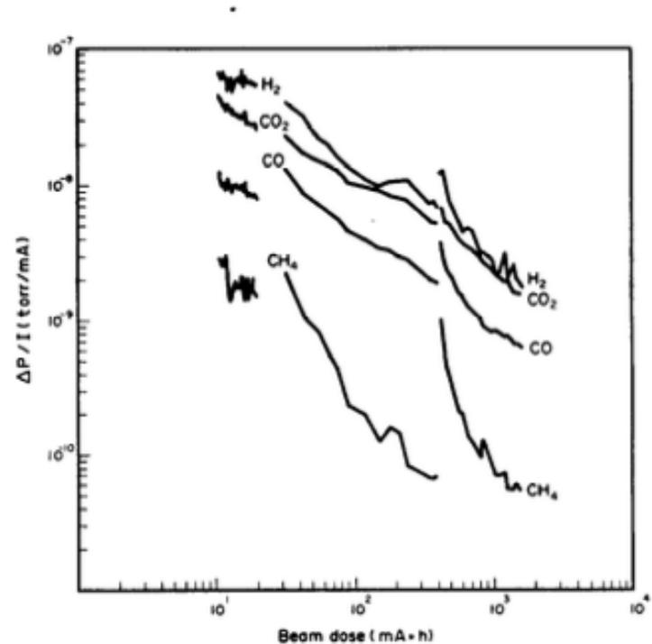
Figure 4. The specific partial pressure rise  $\Delta P/I$  as a function of the beam dose for  $H_2$ ,  $CH_4$ ,  $CO$  and  $CO_2$  for the first series of measurements—unbaked.
