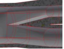
Remaining issue: difficult to dissipate the heat around the RF finger
