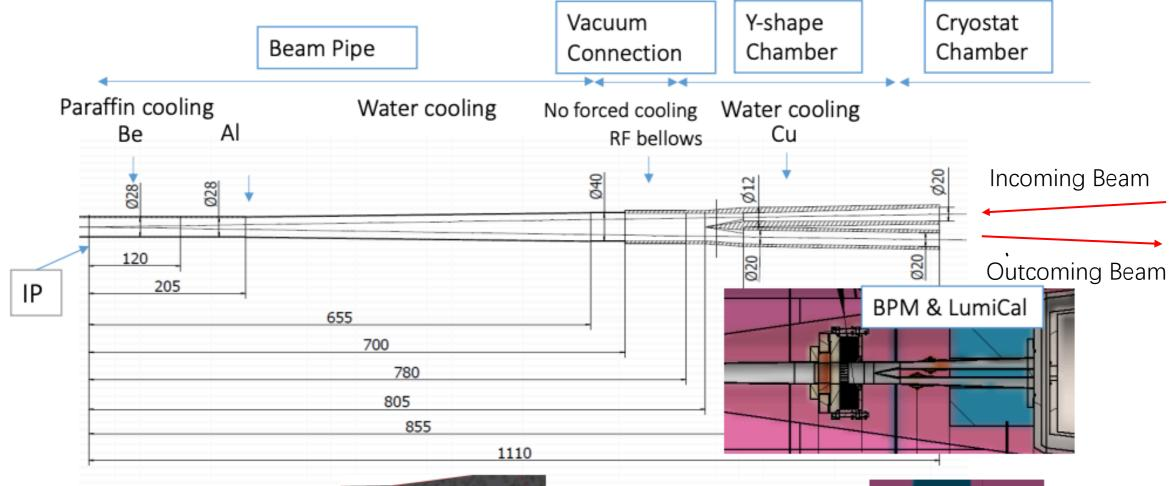
Asymmetric design to prevent direct hitting of synchrotron radiation photons
