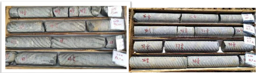
G04钻孔奥陶系砂岩部分岩芯 (IP3) The Ordovician sandstone cores in G04 hole (IP3)
