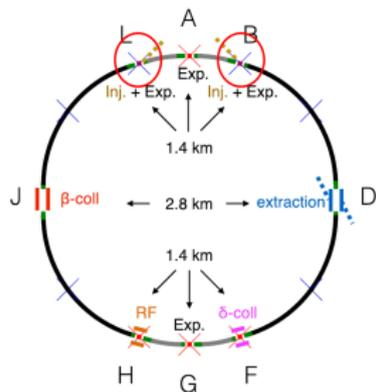
Collision optics LSS-PB-EXP  $\beta^* = 3.0\text{m}$
