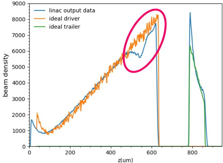
Even assuming the beam is ideal at the exit of e- gun, the beam profile is still not the same as we expected at the linac exit.
