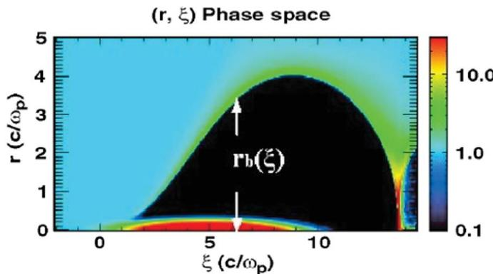
$$\text{The equation of boundary: } r_b \frac{d^2 r_b}{d \xi^2} + 2 \left[ \frac{dr_b}{d \xi} \right]^2 + 1 = \frac{4 \lambda(\xi)}{r_b^2}$$
