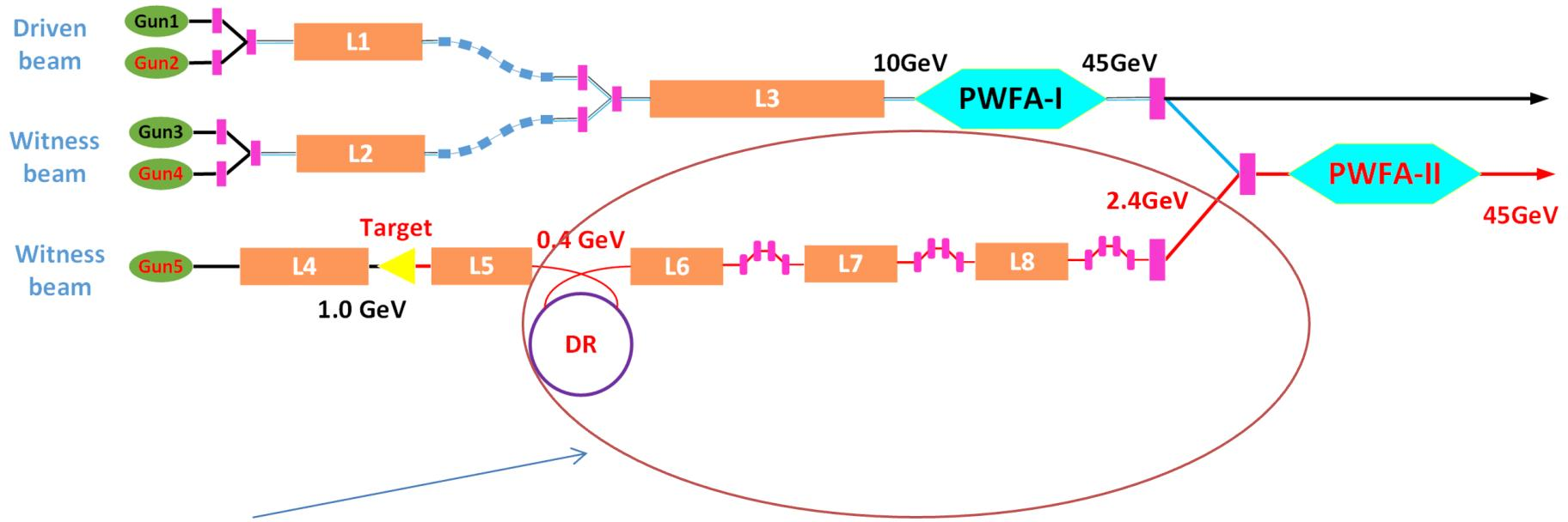
1. Transverse emittance cooling:  $2400\text{mm.mrad} \rightarrow 20\text{mm.mrad}$
