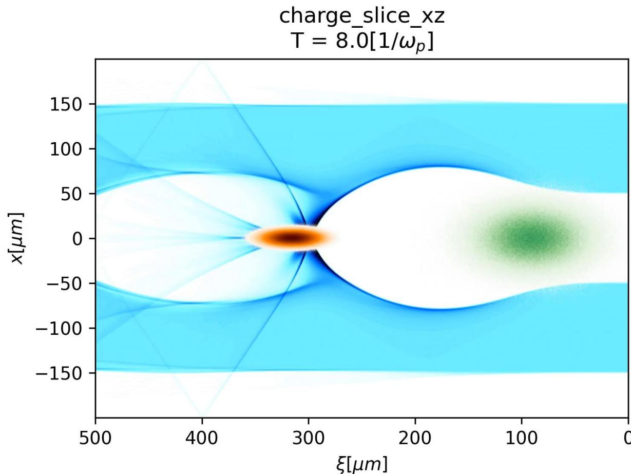
Gradient~5GV/m, Efficiency >30%, Energy Spread~1.5%
