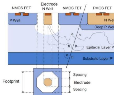
Schematic cross section of a CPS pixel
