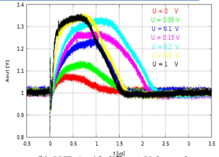
(b) OUT\_A with different Vpluse voltage
