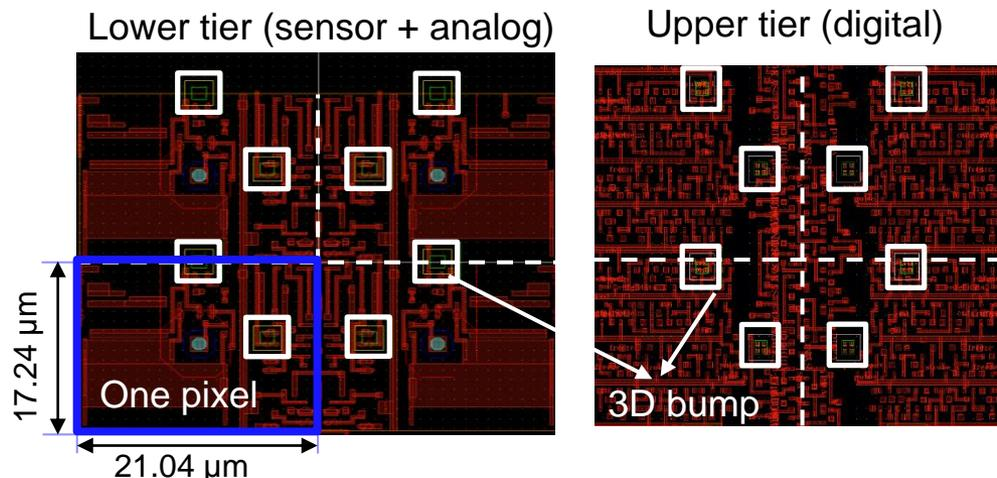
The lower tier can be either SOI or CMOS pixel sensor
