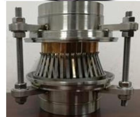
Mould of contact fingers adjustment
