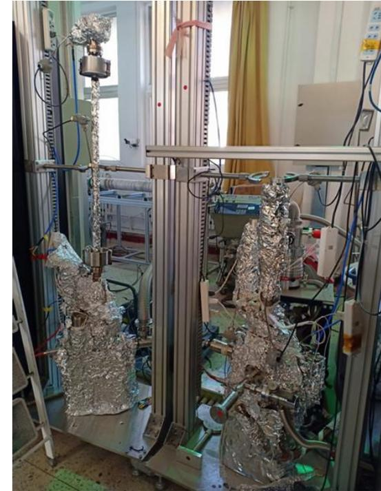
A high pure hydrogen (99.999%) is introduced by the injection valve, the gas passes through the coated pipe and is absorbed by the NEG film. The P2/P1 ratio is measured by the pressure gauges, which is related to the average sticking probability and pumping speed of the pipe walls.
