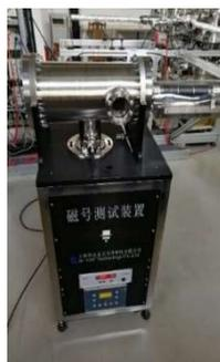
The test bench of the FLUX concentrator
