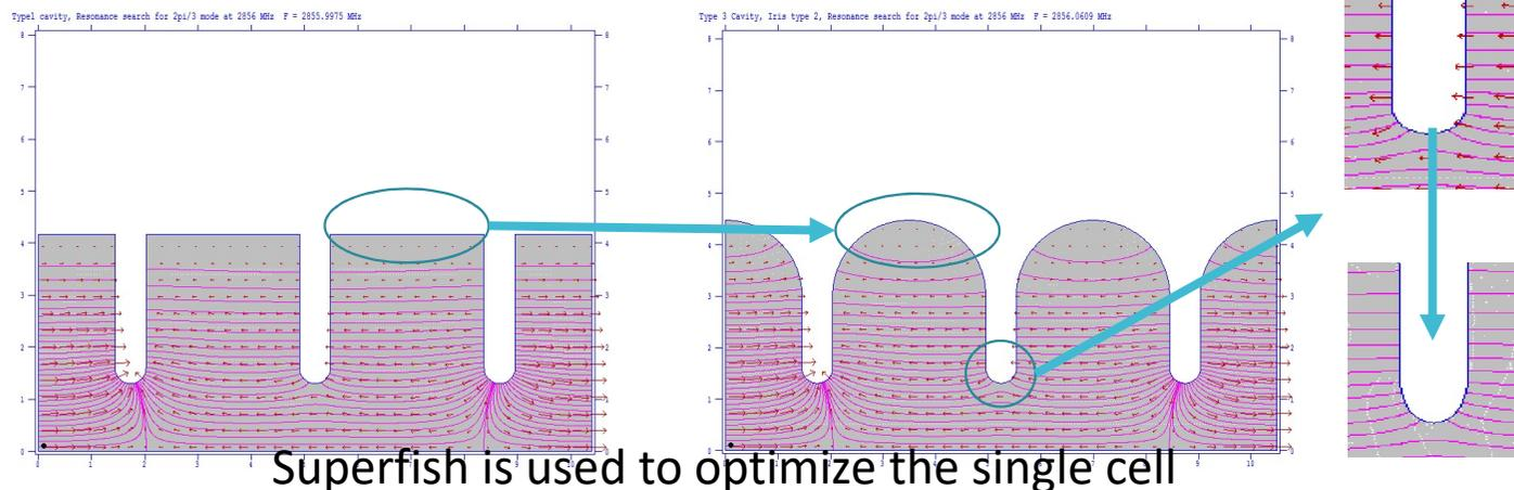
Superfish is used to optimize the single cell
