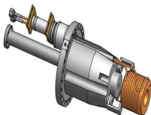
The mechanical design of FLUX concentrator
