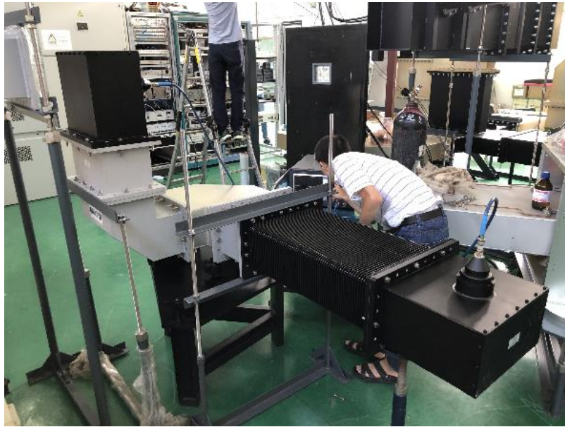
Cold test for waveguide system
