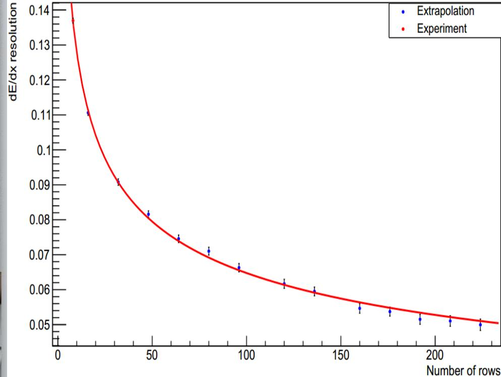
**Experimental study result using laser and expanded to CEPC TPC**
