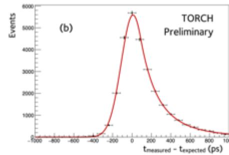
Separating  $\pi/K$  at 10 GeV/c over 10 m ( $\Delta_{\text{TOF}} = 35 \text{ ps}$ ) requires  $\sigma_{\text{TOF}} \approx 10-15 \text{ ps}$ . Aim at  $\sigma_{1y} = 70 \text{ ps}$  with  $N_y = 30$
