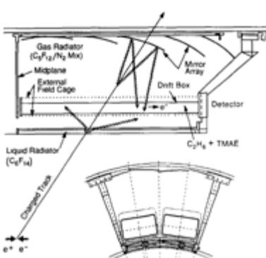
Fig. 1. Schematic of the SLD barrel CRID.
