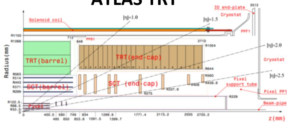
380,000 straw 4 mm dia. (Xe/CO<sub>2</sub>/O<sub>2</sub>) in polyethylene foam
