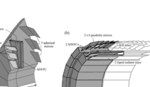
Fig. 2. Main components of the RICH detectors. (a) Forward RICH. (b) Barrel RICH.
