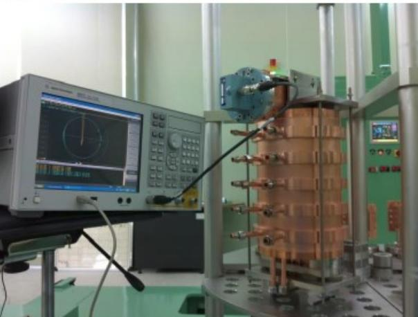
RF Inspection by Network Analyzer
