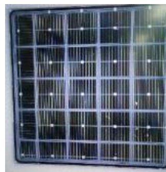
IHEP-NDL LGAD-V2 Pixel size 1.3 \times 1.3 mm 2
