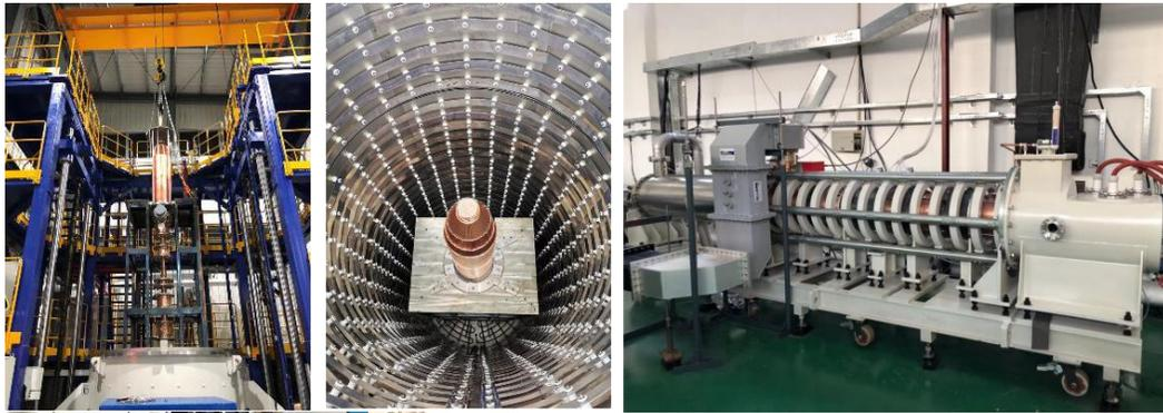
On March 10, 2020, the first CEPC650Mhz klystron output power has reached pulsed power of 800kW (400kW CW due to test load limitation), efficiency 62% and band width>+0.5Mhz.
