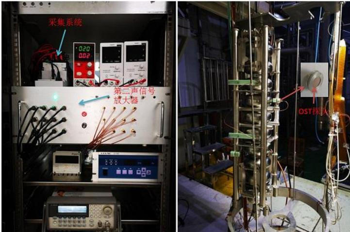
SC cavity vertical test temperature monitor system established
