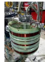
Helmholtz coil for cavity vertical test
