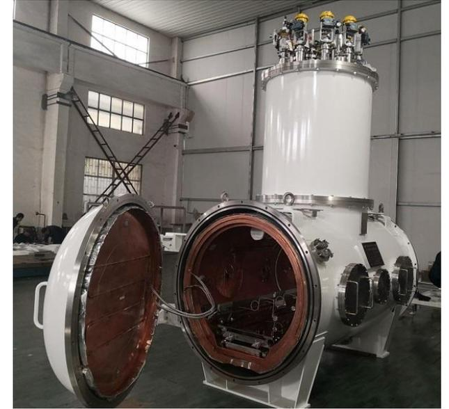
General superconducting cavity test cryomodule in IHEP New SC Lab
