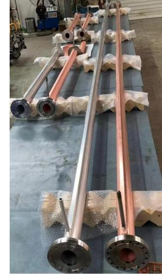
Two 6m long vacuum chambers both for copper and aluminum
